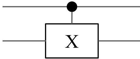
$$\begin{aligned} |0x\rangle &\rightarrow |0x\rangle \\ |10\rangle &\rightarrow |11\rangle \\ |11\rangle &\rightarrow |10\rangle \end{aligned}$$
