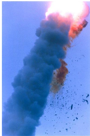
Explosion of first Ariane 5 flight, 1996 (Overflow during data conversion)
