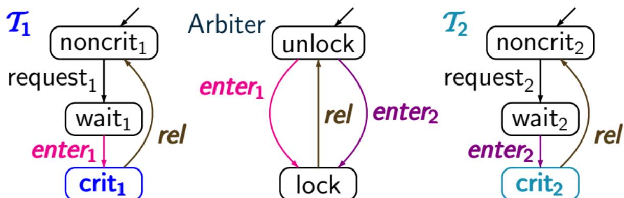
$\mathcal{T}_1$  and  $\mathcal{T}_2$  compete to communicate with the arbiter by means of the actions **enter<sub>1</sub>** and **enter<sub>2</sub>**, respectively
